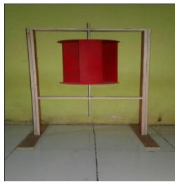
Gambar 2.4. Kincir Angin sumbu vertical tipe sudu 90^\circ 4sudu
